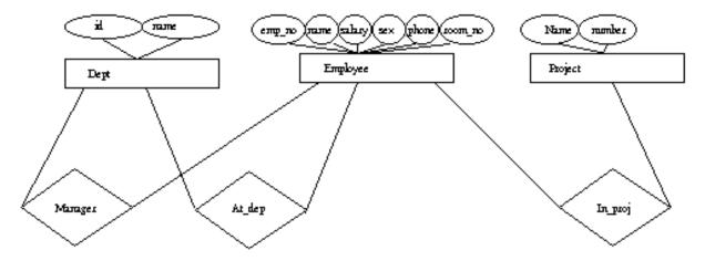
Figure 3.1: Company Entity-Relation Diagram
