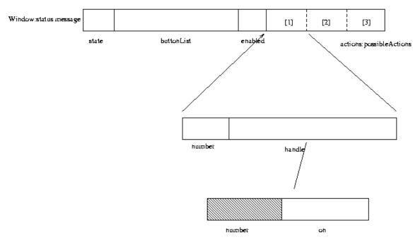
Figure 4.3: Bytes of a Window:status Message
