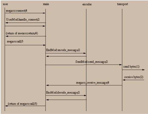
Figure 3.2: MG Startup Call Flow
