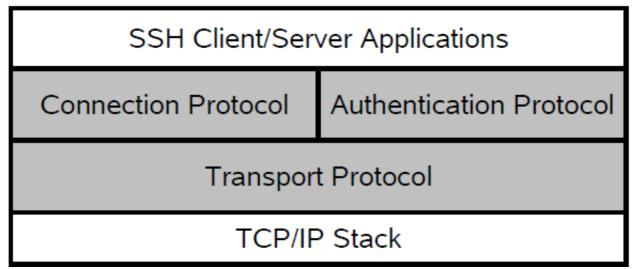
Figure 1.1: SSH Protocol Architecture
