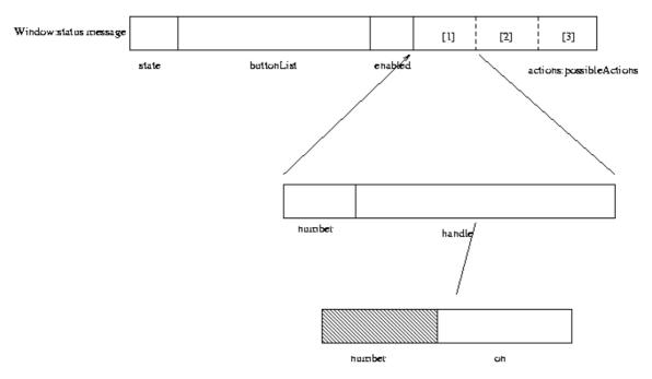
Figure 4.3: Bytes of a Window:status Message
