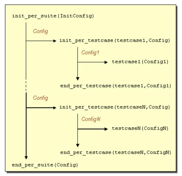
Figure .2: Config data flow in the suite.
